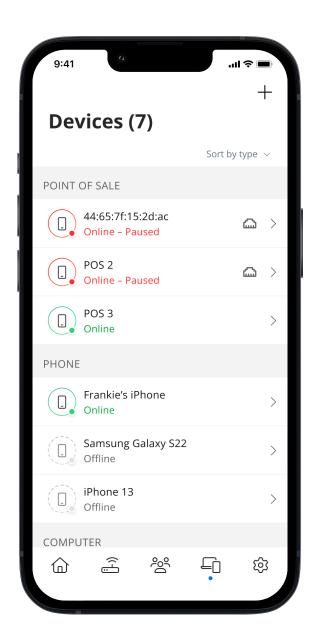
The Devices list allows you to manage the devices connected to your network. Tap on a device to enable/disable internet access or to see additional details including:
