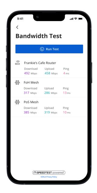
The easiest way to run a bandwidth test is to tap **Networks** and then tap the **Bandwidth Test** icon. Then simply tap the **Run Test** button.
