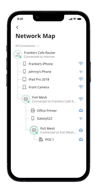
The Network Map provides a topological view of your network. To view the Network Map, tap **Networks** on the dashboard. Next, tap Network Map to view devices connected to your system. Tap on the Mesh icon to view performance information and devices connected at that Mesh unit.
